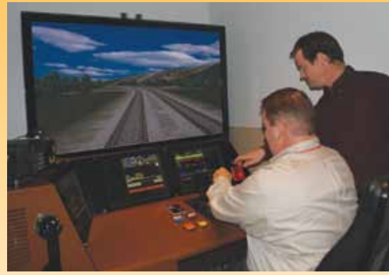
A Technical Training Center instructor points out the display for BNSF's positive train control system on a locomotive training simulator.
