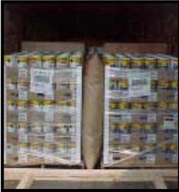
Lading unitized with stretch wrap to the pallet and braced by floor blocking and DID bag
