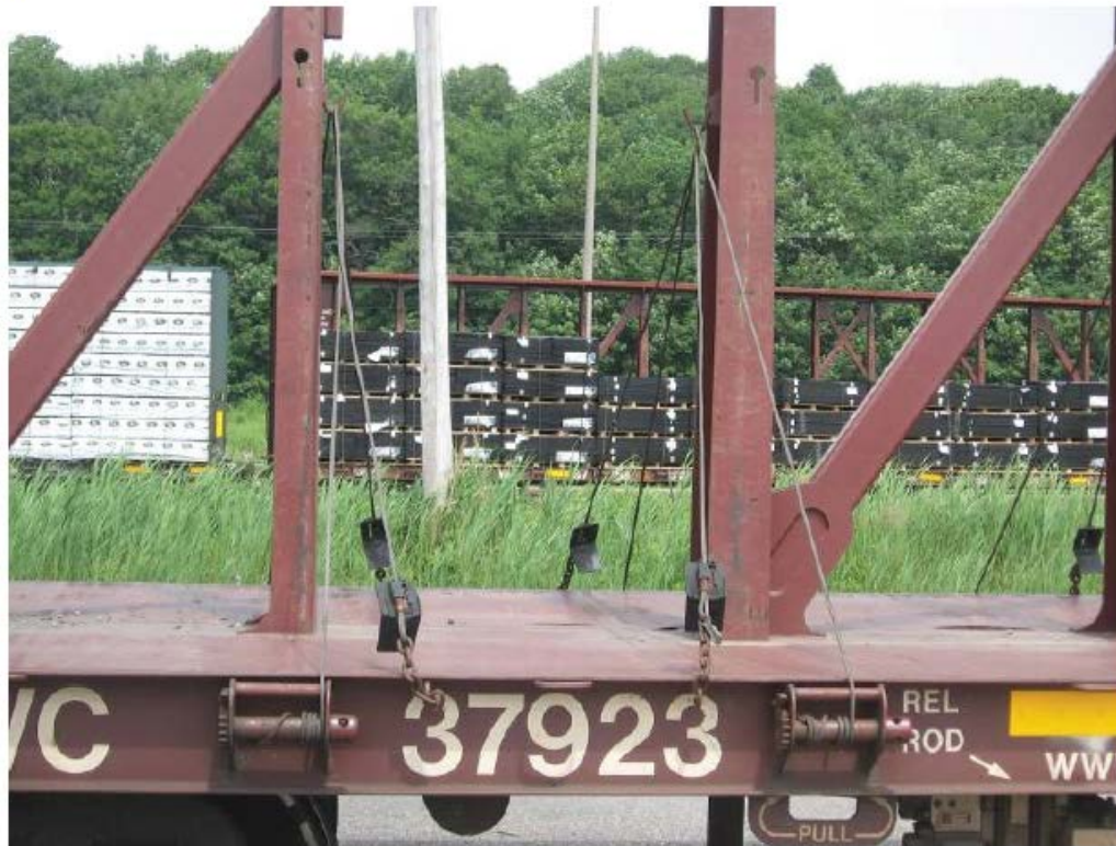
Fig. 22.5 Properly secured cable for empty movement of railcar
