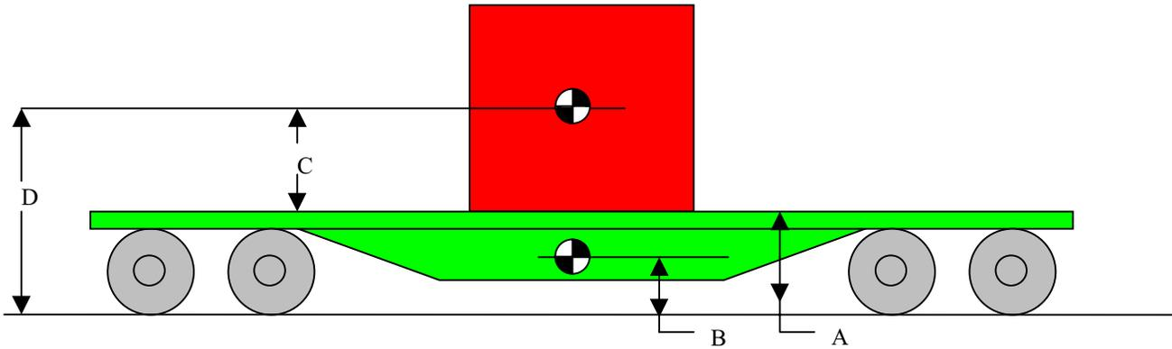
The following information is necessary to determine the combined center of gravity of a loaded railcar.
